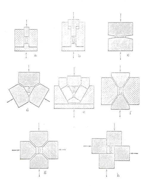
Fig. 1. Various types of high-pressure chambers
